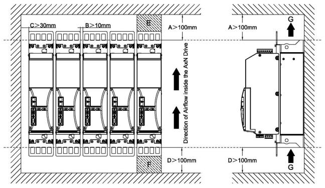
Installation Spacing of AxN Size2 Series Drive
