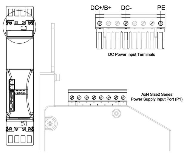
**Step 3: Insert Wires into Corresponding Terminals**
