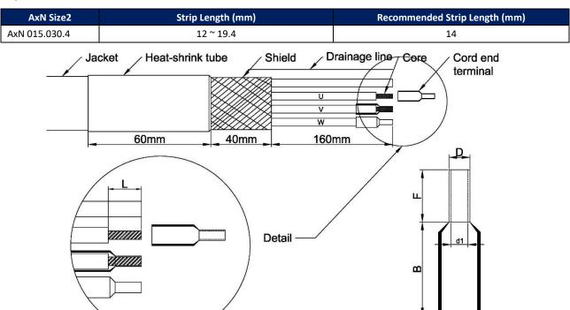
Step 7: Connect the PE wire with Shield
