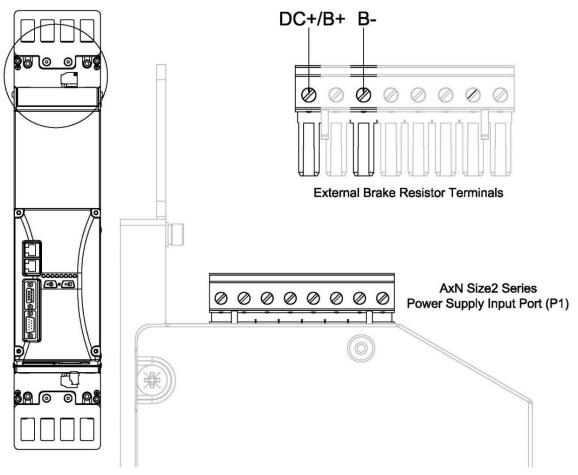
**Step3: Insert Wires into Corresponding Terminals**
