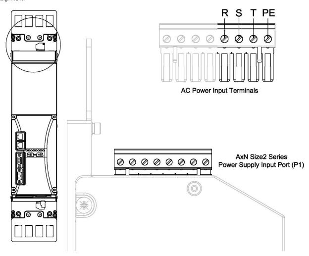
**Step 4: Insert Wires into Corresponding Terminals**
