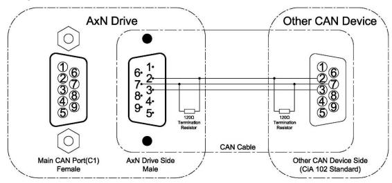
Note: Only the first and the last CAN node device should use a  $120\Omega$  terminal resistor.
