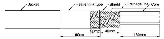
Step 6: Make the Phase Wires
