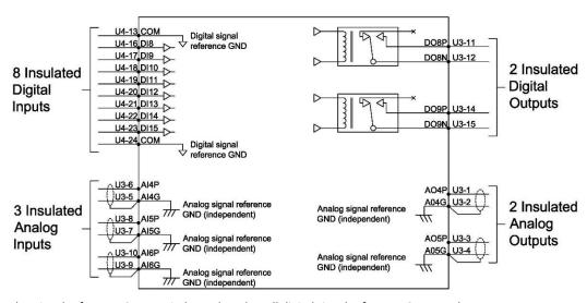
**NOTE:** All analog signal reference GND are independent, but all digital signal reference GND are the same.
