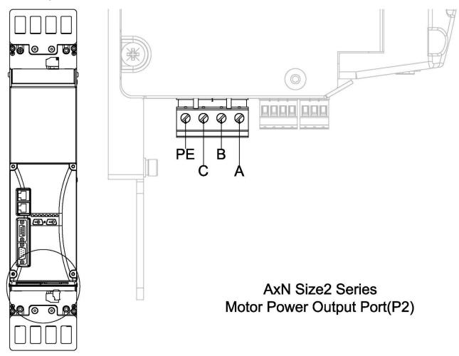
**Step 2: Insert Wires into Corresponding Terminals**
