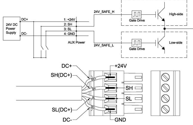
Apply 24 (±15%) Vdc power supply on the Pin 2: SH and Pin 3: SL with porper control system to enable the STO Function.
