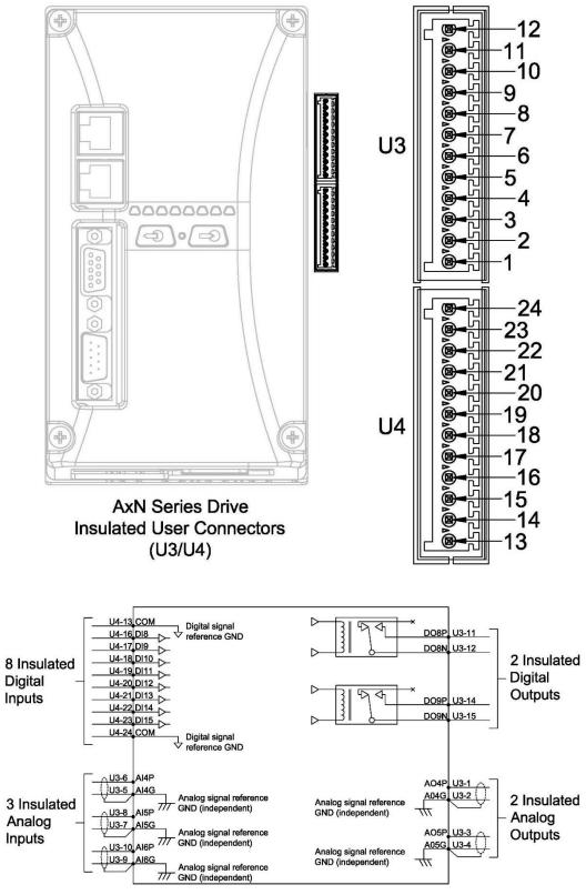
NOTE: All analog signal reference GND are independent, but all digital signal reference GND are the same.
