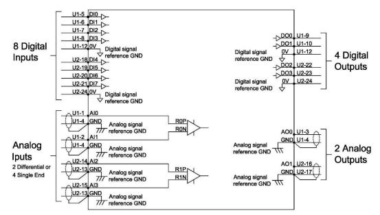
NOTE: All analog signal reference GND are the same, and all digital signal reference GND are the same.
