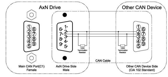
Note: Only the first and the last CAN node device should use a 120  $\!\Omega$  terminal resistor.
