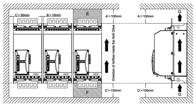
Installation Spacing of AxN Size4 Series Drive
