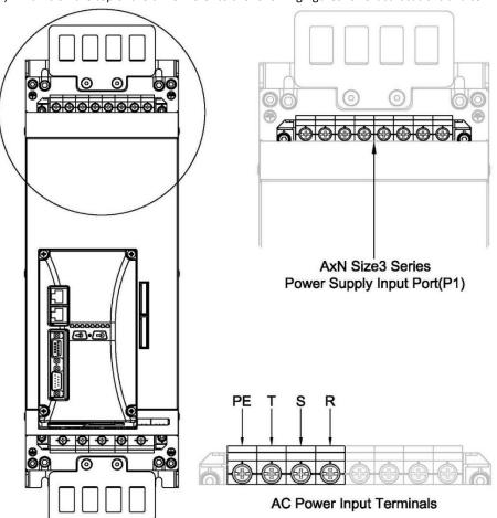
**Step 4: Insert Wires into Corresponding Terminals**
