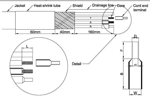
Step 7: Connect PE wire with Shield
