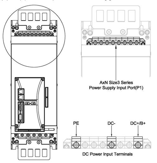
Step 3: Insert Wires into Corresponding Terminals
