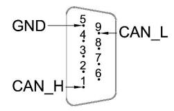
Note: CANopen pin assignment on S1 connector does NOT meet CiA 102 Standard.
