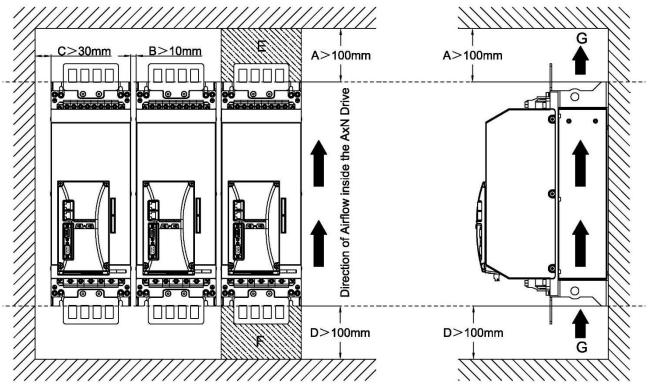
**Installation Spacing of AxN Size3 Series Drive**
