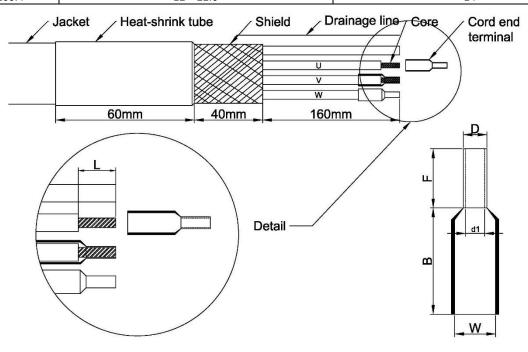
Step 7: Connect the PE wire with Shield
