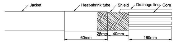
Step 6: Make the Phase Wires
