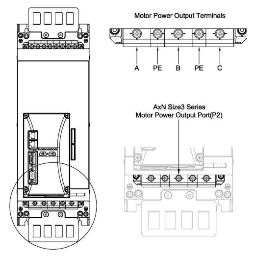
**Step 2: Insert Wires into Corresponding Terminals**
