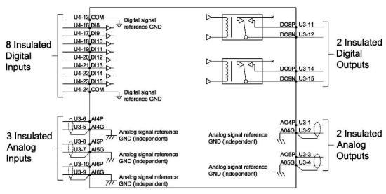
NOTE: All analog signal reference GND are independent, but all digital signal reference GND are the same.
