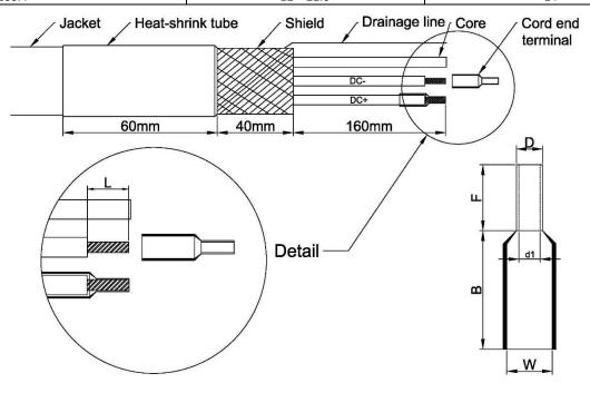
Step 7: Connect PE wire with Shield
