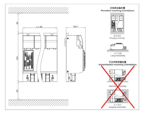
1) For proper air circulation, at least 60 mm clearance must be available above and below the module.
