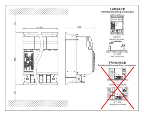
1) Preference is given to vertical suspension installation, secondary placement horizontal placement; 2) For proper air circulation, at least 60 mm clearance must be available above and below the module.
