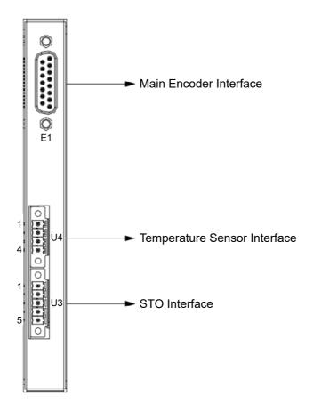
The control platform of AxN-DC drive supports SinCos encoder, Endat 2.2 encoder, Resolver, digital incremental encoder, Nikon encoder and, Tamagawa absolute encoder and Hiperface encoder.
