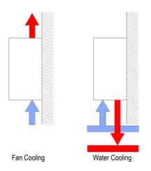
Depending on the structure, there are two cooling methods:
